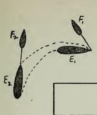
$E_1$  "Edith" reversing and backing to her starboard eases strain and assists  $F_1$  "Fearless" in swinging head around with minimum strain on towing hawser.
